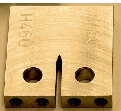
CT specimen 30x28.8x12 mm 3
