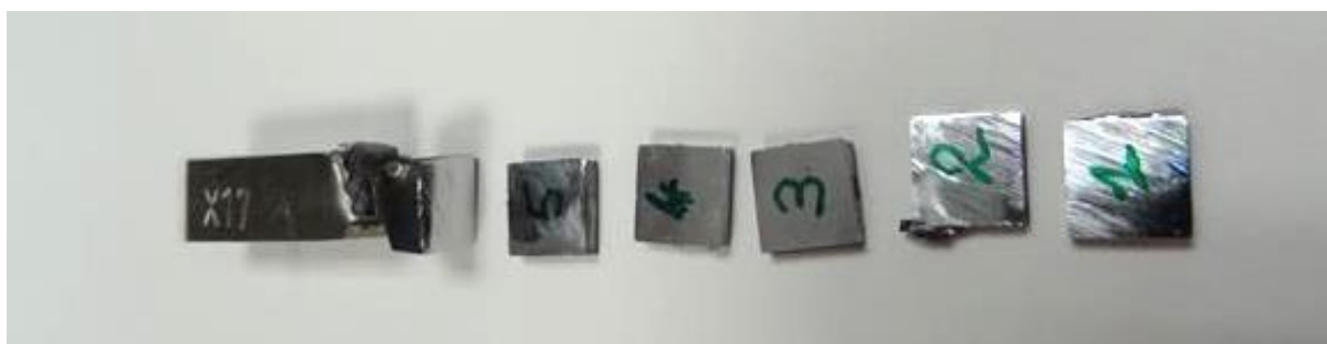
Figure 1. General view of the cut JRQ Charpy-V sample.
