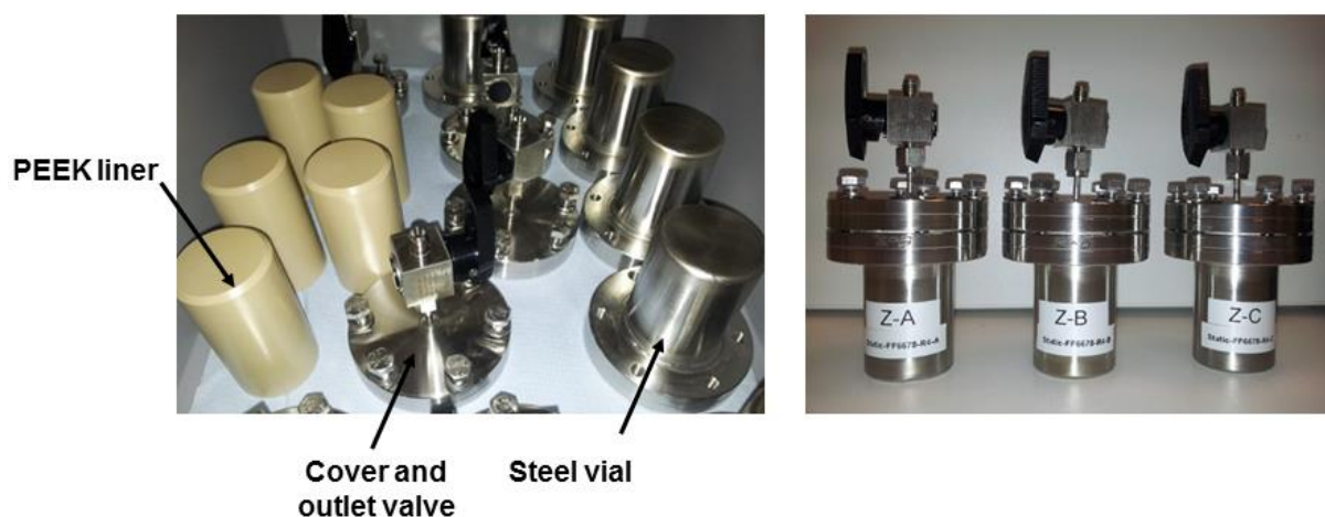
Figure 5. Picture of the static test setups (A) before assembly and (B) after assembly.
