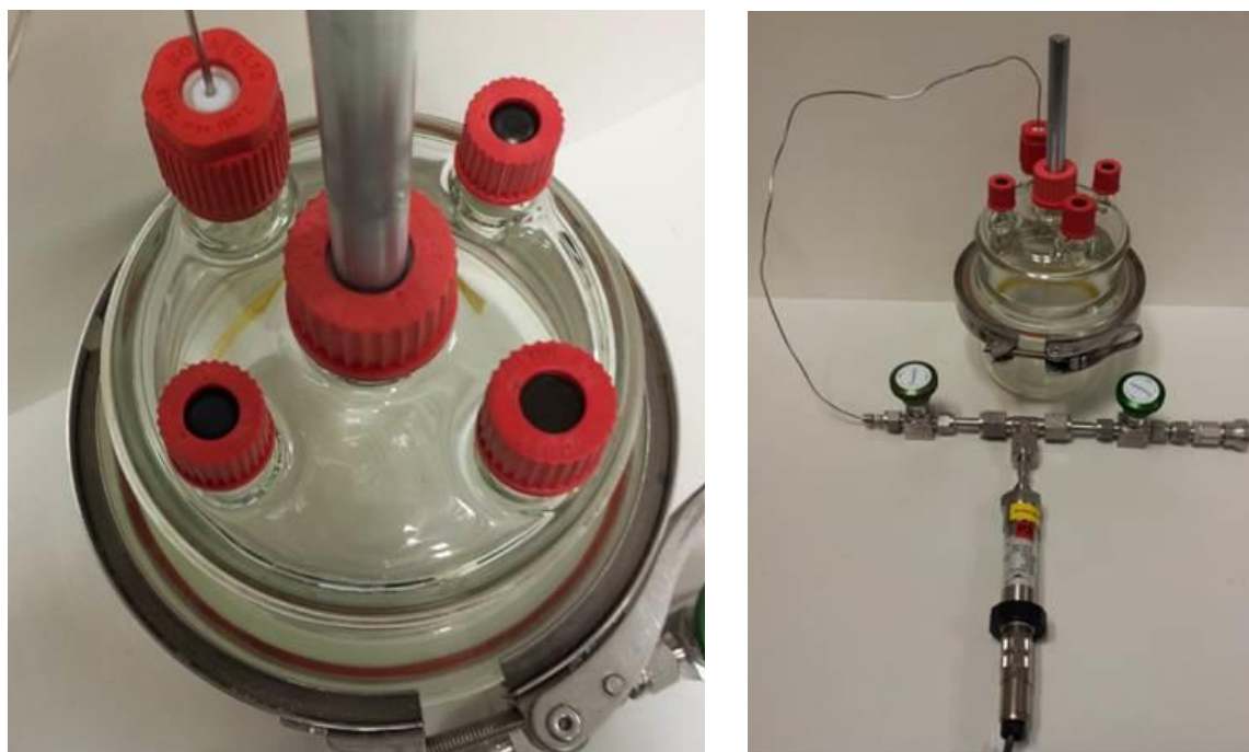
Figure 11. Setup for gas tightness testing of the electrochemical cell.
