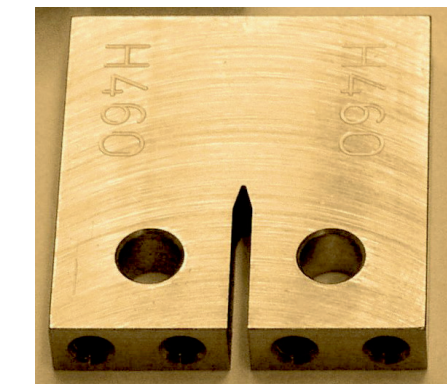
CT specimen 30x28.8x12 mm 3
