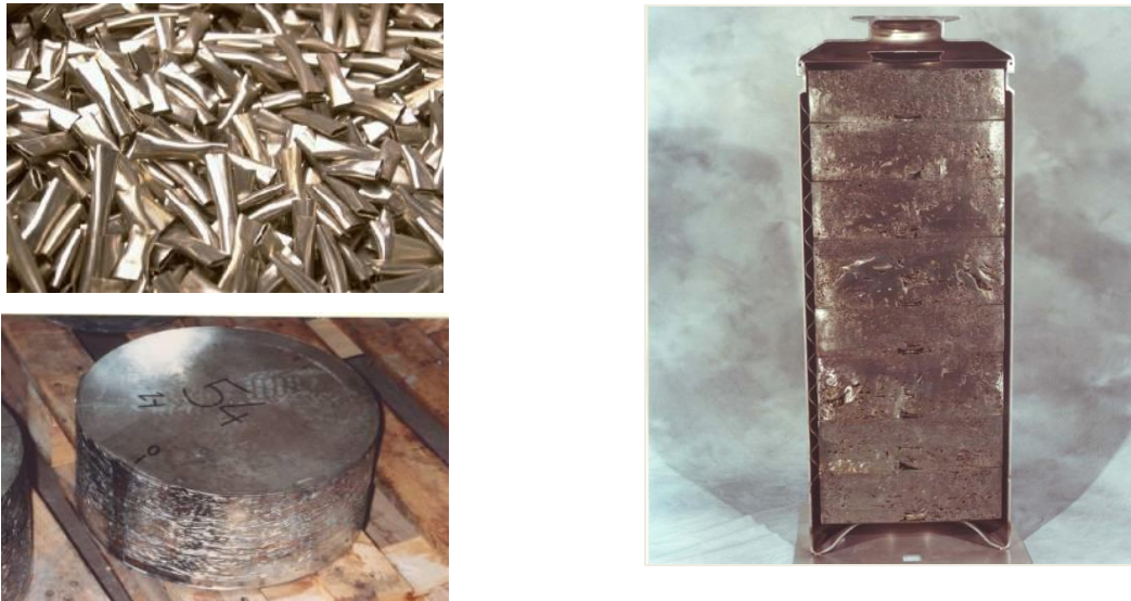
Figure 17: On the left, hulls and galette of press compacted hulls and end-pieces; on the right, stack of galettes of press compacted waste in CSD-C waste package (Areva NC photographs)
