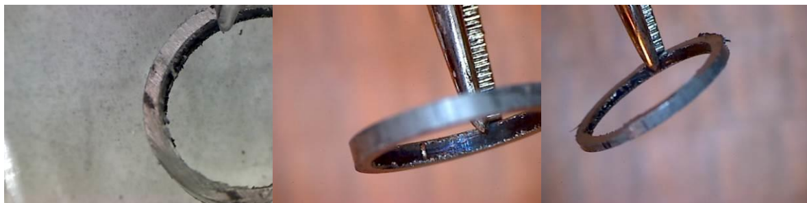
Figure 7: Black/blueish precipitates seen on the inner surface of the irradiated Zircaloy-4 cladding.
