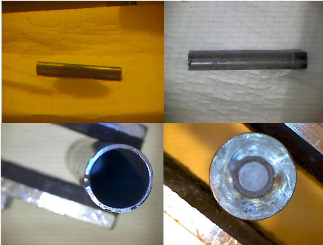
Figure 1: The upper two pictures show the whole irradiated Zircaloy-4 plenum specimen available at KIT-INE. The lower left picture shows the bottom half of the specimen, where the plenum was cut from the fuel rod segment whereas the lower right picture shows the end cap of the plenum specimen.
