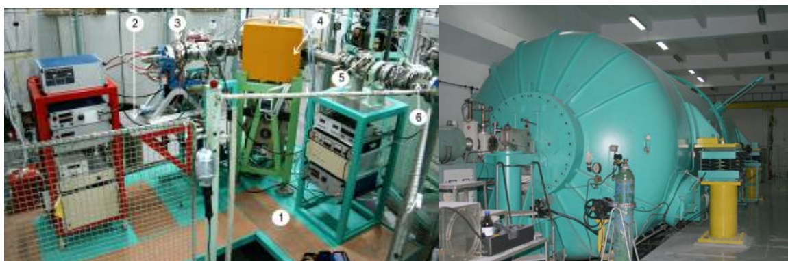
Figure 2.8.6 and Figure 2.8.7. Left: the Injector deck of the 9 MV tandem AMS facility in Bucharest: 1) Injector platform polarized at -100 kV; 2) second platform polarized at -30kV in respect to the first platform; 3) the ion source (40 NC-SNICS ); 4) 90 0 analyzing magnet; 5) slits and retractable Faraday cup; 6) pre-acceleration NEC tubes. Right: the tandem 9 MV FN accelerator.
