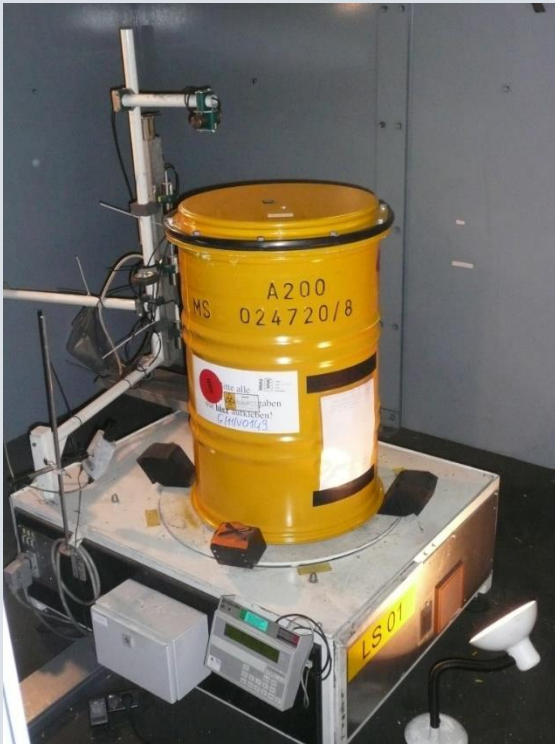
dose rate measurement, weight check and photo documentation
