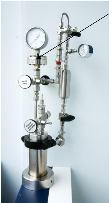
Figure 2 Autoclave with gas mouse attached. The connection requires improvement in order to allow optimum sampling and avoid transfer of contamination to the analytical glove box.
