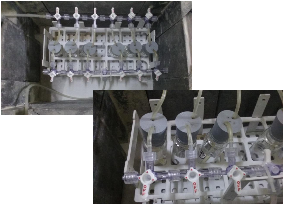
Figure 4 View of the six glass bottles used in the leaching tests
