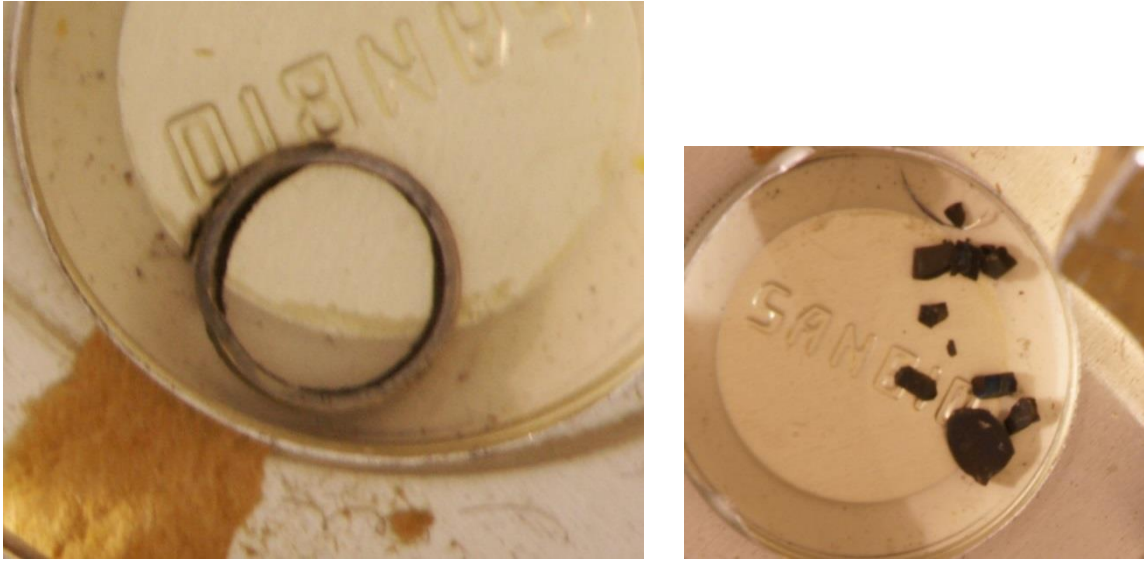
Figure 1(left): Dark film on inner surface seen after the first acid cleaning. Little difference is seen after the second acid cleaning; (right): pieces of fuel after defueling.
