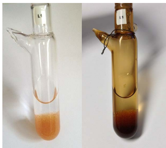
Figure 21. Sample vials filled with anion exchange resins and water, before (left) and after irradiation (right).
