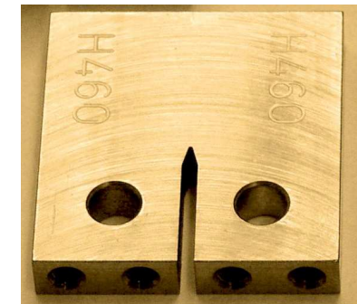
CT specimen 30x28.8x12 mm 3
