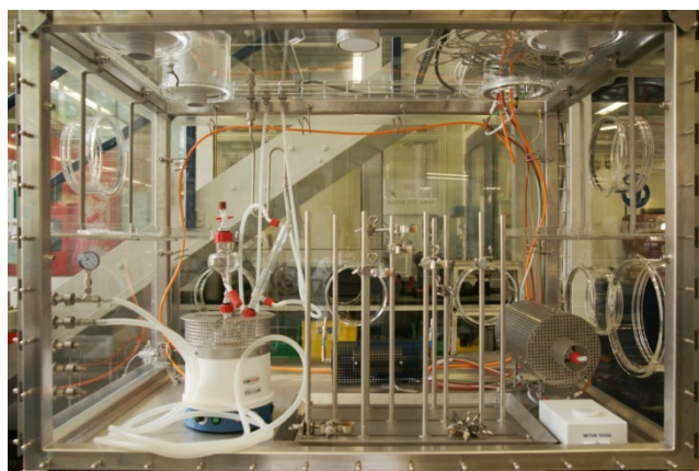
Figure 6.3: Horizontal view with the heating element and furnace with the additional shielding for protection against hot areas during operation of the furnaces
