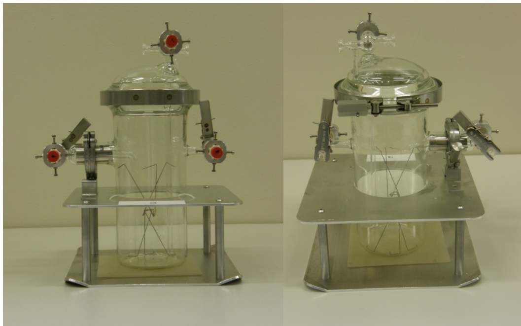
Figure 8.4: CAST leaching container placed in a rack with tools for manipulation in the HCL (front side – left and back side –right)
