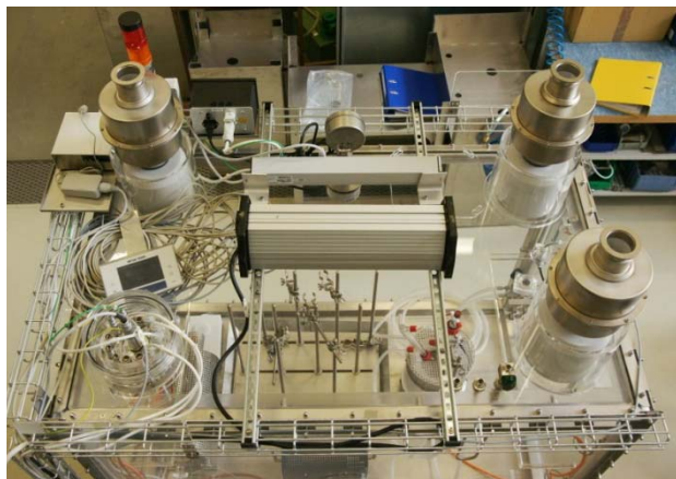
Figure 6.2: Photograph showing the additional work on the glove box roof: glove box (GB) filter system and GB lighting placed on top
