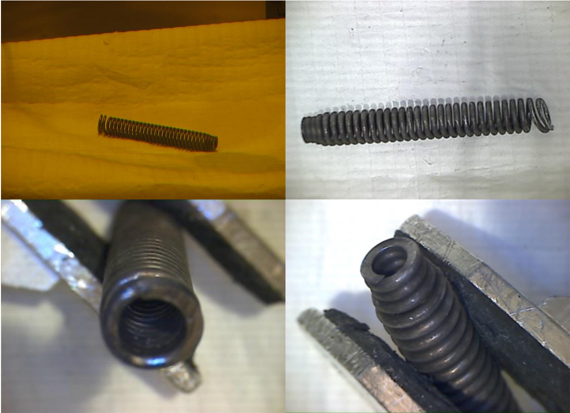
Figure 2: Irradiated stainless steel plenum spring used for the dissolution experiments.
