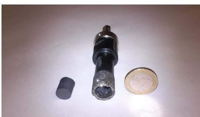
Figure 5 (Above). Graphite core 11 mm x 12 mm ( \text{Ø} x H) and diamond core drill 14 mm \text{Ø} .
