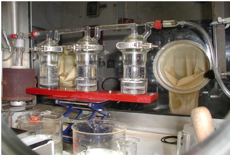
Figure 4: Experimental setup used for the quantification of total ^3\text{H} and ^{14}\text{C} inventories in i-graphite.
