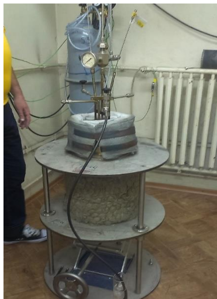
Figure 2 Static autoclave used to oxidize the non-irradiated Zy-4 samples
