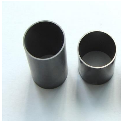
Figure 23 Oxidised Zy-4 tube (left), oxidized Zy-4 tube cut at one end (right)
