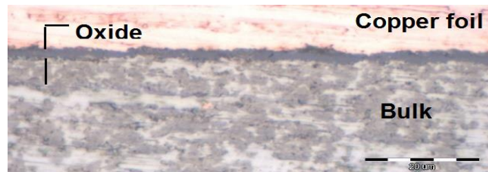
Figure 14 Oxide layer thickness measured by optical microscopy (magnification x1000)
