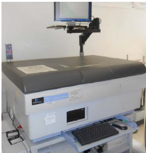
Figure 5: Tri-Carb analyzer, ^{14}\text{C} detection limit: 0.02 Bq/mL
