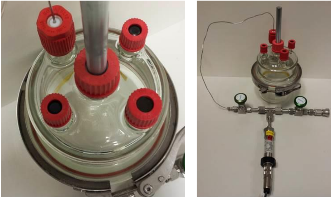
Figure 11. Accelerated corrosion test cell setup.
