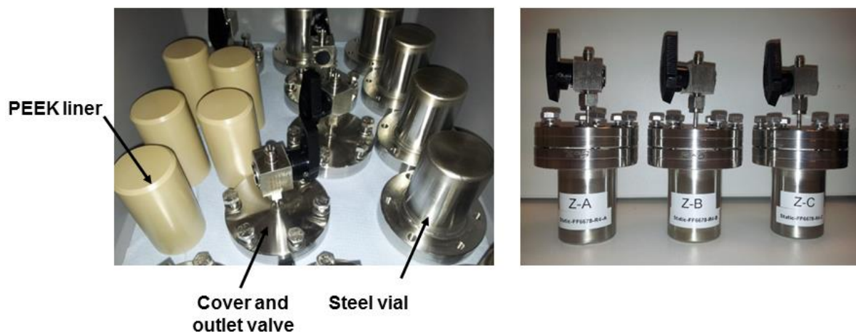
Figure 5. Photographs of the static test setups (A) before assembly and (B) after assembly.
