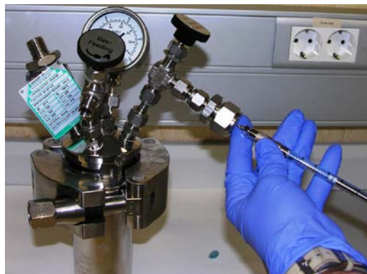
Figure 7. The gas sample extraction by a syringe
