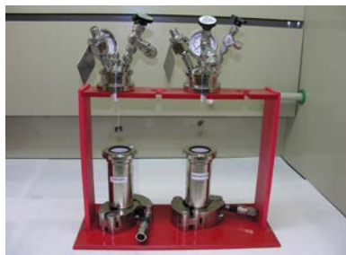
Figure 6. Leaching containers for deionized water and granitic-bentonite water
