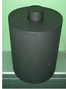
Figure 2. Pressing Tool of 2 cm diameter
