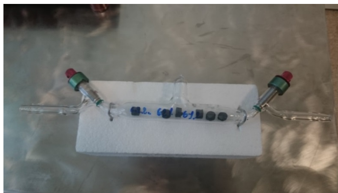
Figure 6: Graphite samples sealed in a glass vessel
