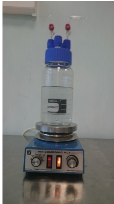
Figure 5: Graphite sample submerged in sodium hydroxide solution placed on a stirrer
