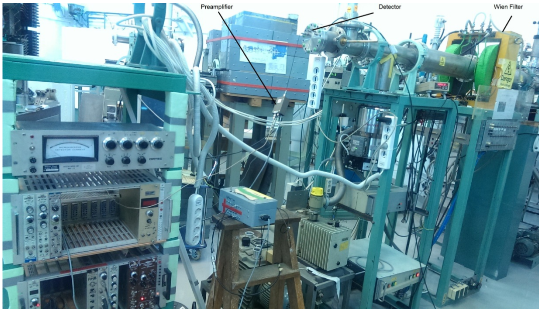
Figure A4: Preamplifier, Detector and Velocity filter set up.
