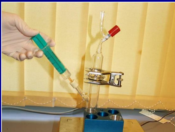
1-3 mL of NaOH prepared by acid in vacuum cell
