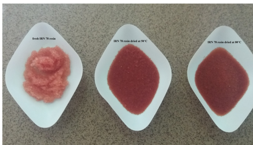
Figure 12. The resin samples used in the sorption tests at RATEN-ICN
