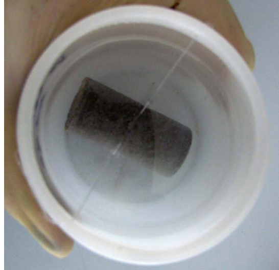
Figure 4. Sample of solidified SIER prepared for leaching experiment.
