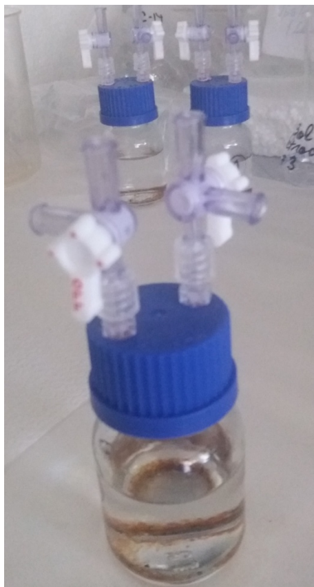
Figure 3. The glass vessels adapted for desorption tests
