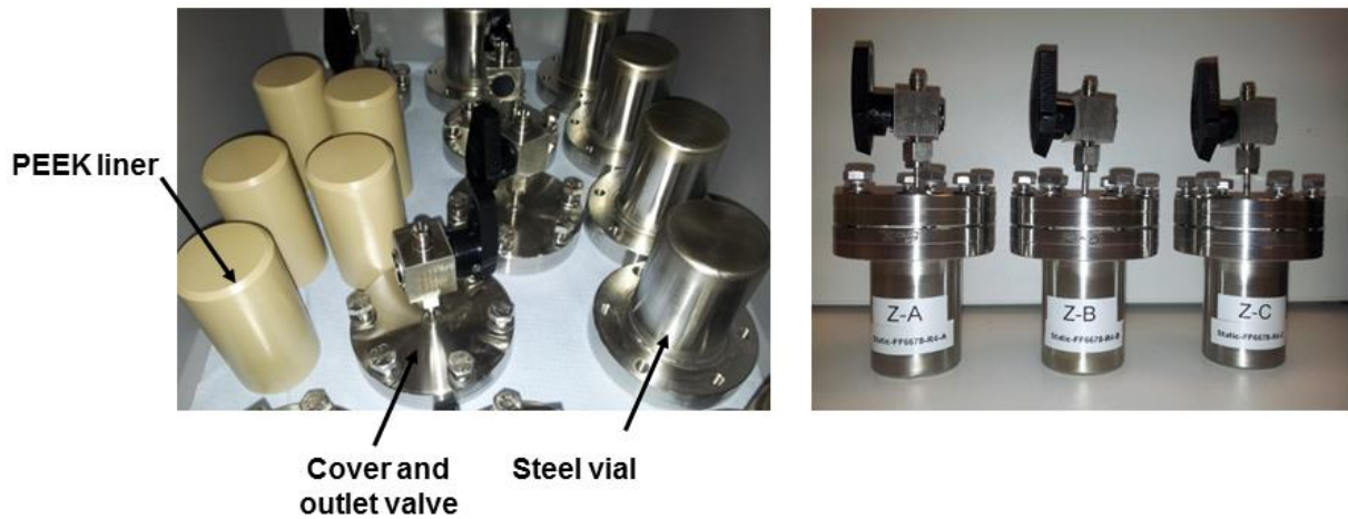
Figure 4. Leaching vials used for the leaching tests at SCK•CEN.
